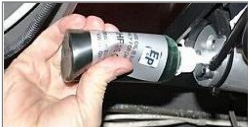
- Refilling of hydraulic oil.
