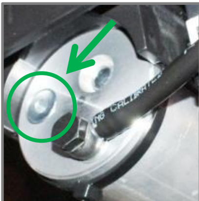
- Oil filling screw in pump.
