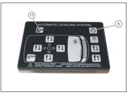
2. Push the *Retract all jacks* button (8) and hold it down until all jacks are fully retracted.
