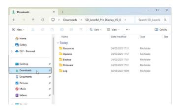
Connect the PC to the Display with a USB-C cable and switch the display on. If everything works you will see USB on the display and in the explorer on the PC you see a new USB drive. If you don't see the USB drive you have probably a charge-only cable. These cables have only charge wires but not the wires to communicate. If you want to test this, connect a other device like a phone with the cable an check if this is detected and seen by the PC.
